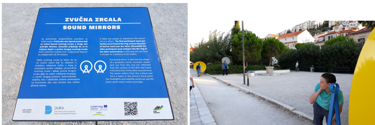
Figure 6: An outdoor activity in Dubrovnik, Croatia, demonstrating sound transmission via two parabolic mirrors: the mirrors are made of yellow metal disks and their foci are highlighted with blue circular rings
